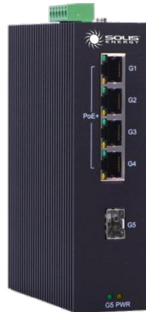
The PoE-4-48, manufactured by Solis Energy, is an unmanaged, hardened, industrial-grade switch designed to reliably connect PoE devices in harsh environments. The PoE-4-48 features four 802.3af/at Gigabit PoE ports and one SFP uplink which allow it to handle cutting-edge high-power and high-bandwidth devices.
